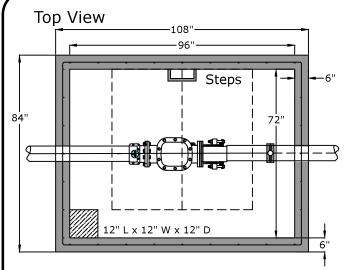
Sensus or approved equal compound or turbo meter with Smith-Blair 913 Flanged Coupling Adapter Meter Supplied by H.V.U.D. at developers expense By pass line to be same size as main line
